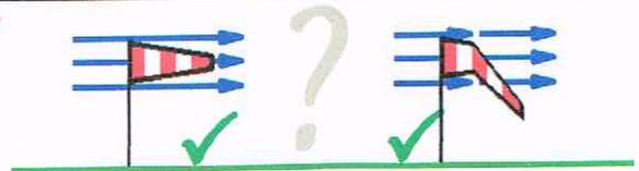
**LE SENS DU VENT AU SOL PERMET DE DÉTERMINER LE SENS DE POSÉ.**
